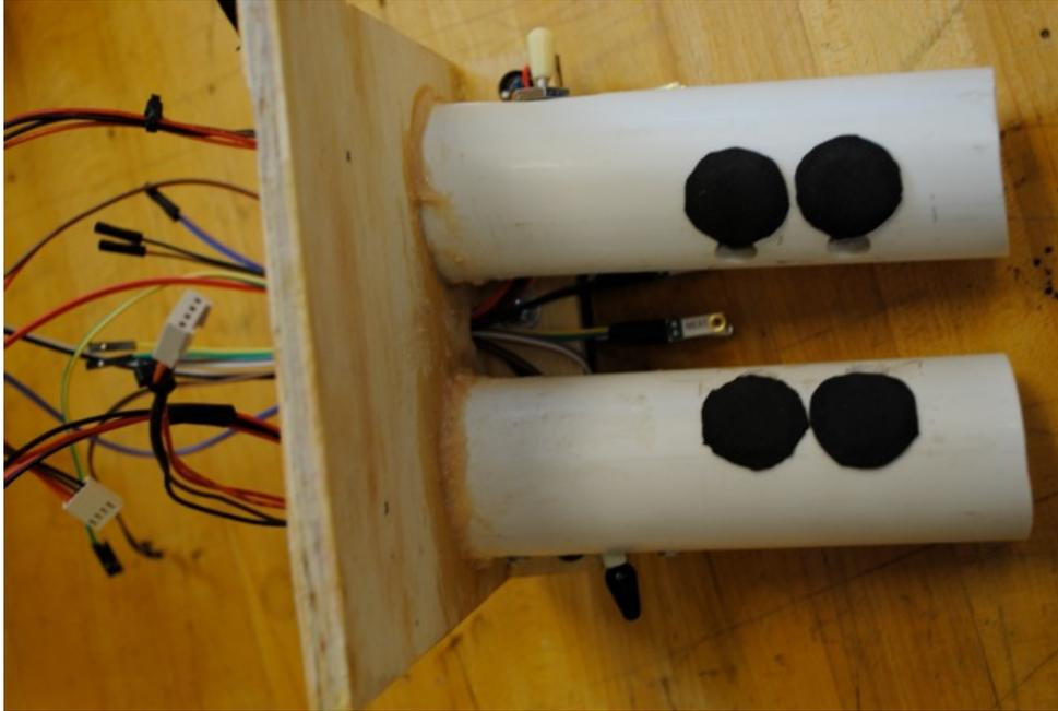
**Figure 2:** FSRs mounted to PVC pipes with neoprene pads
