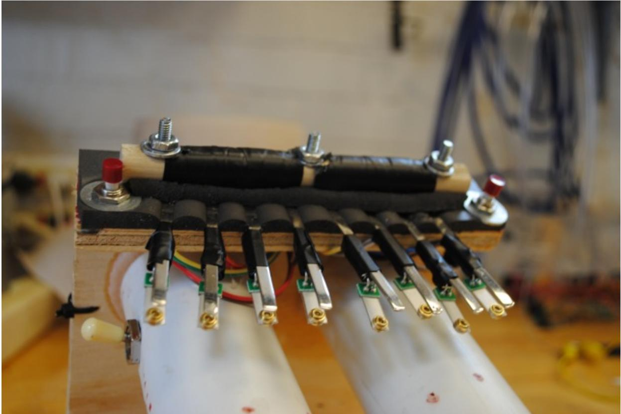
**Figure 1:** Piezo sensors mounted to kalimba keys
