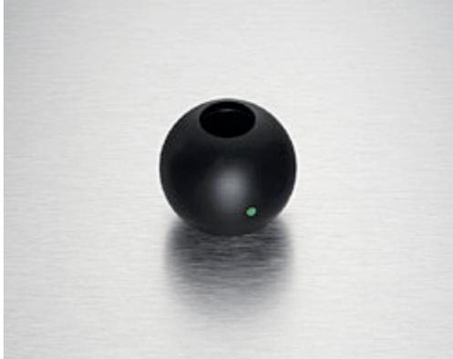
With the DPA Acoustic Pressure Equalisers you are able to modify the frequency response of the 4003 or 4006. This is done without adding any noise or distortion from EQs because the lift is done acoustically at the diaphragm. The L40B sphere will introduce a presence boost and more directionality at higher frequencies, which in sound color is identical to old legendary microphone types originally used by Decca, only with the much higher degree of naturalness offered by a DPA microphone.
